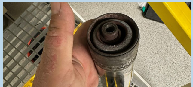
Failed Bearing on Tracking roller
